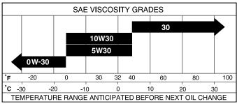
**NOTE:** Although multi-viscosity oils (5W30, 10W30 etc.) improve starting in cold weather, these multi-viscosity oils will result in increased oil consumption when used above 32°F. Check your engine oil level more frequently to avoid possible engine damage from running low on oil.
